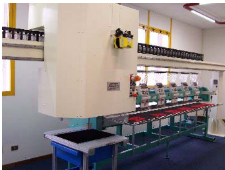
A Bridge Laser (SEIT Laser 4) machine connected with a Tajima multi head embroidery machine.
